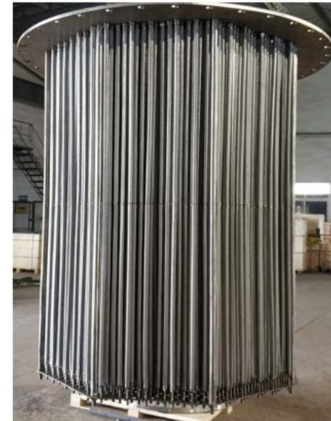
**Stainless Steel tube bundle for 25 m<sup>3</sup>/hr which is placed in 1 m diameter Housing**
